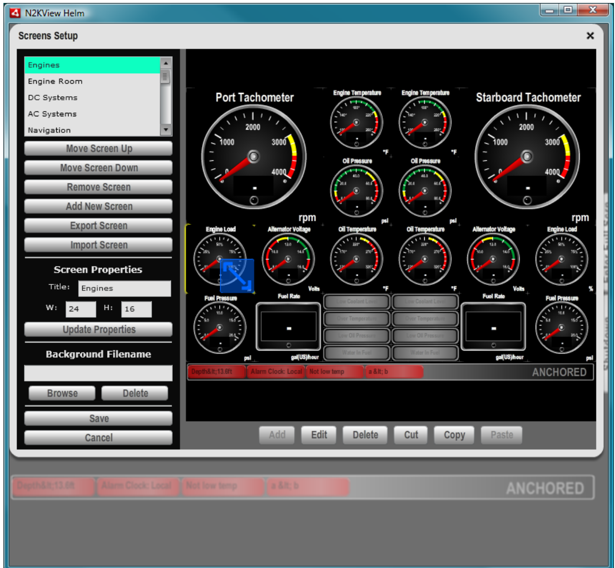
Figure 39 – Screens Setup Screen
