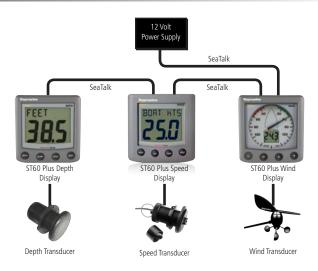
Typical ST60 Plus Depth, Speed and Wind System
